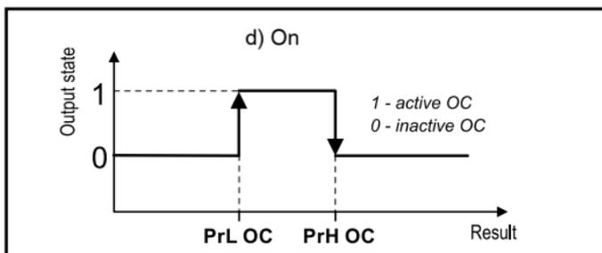
**Fig. 7. Types of OC1 and OC2 output**
