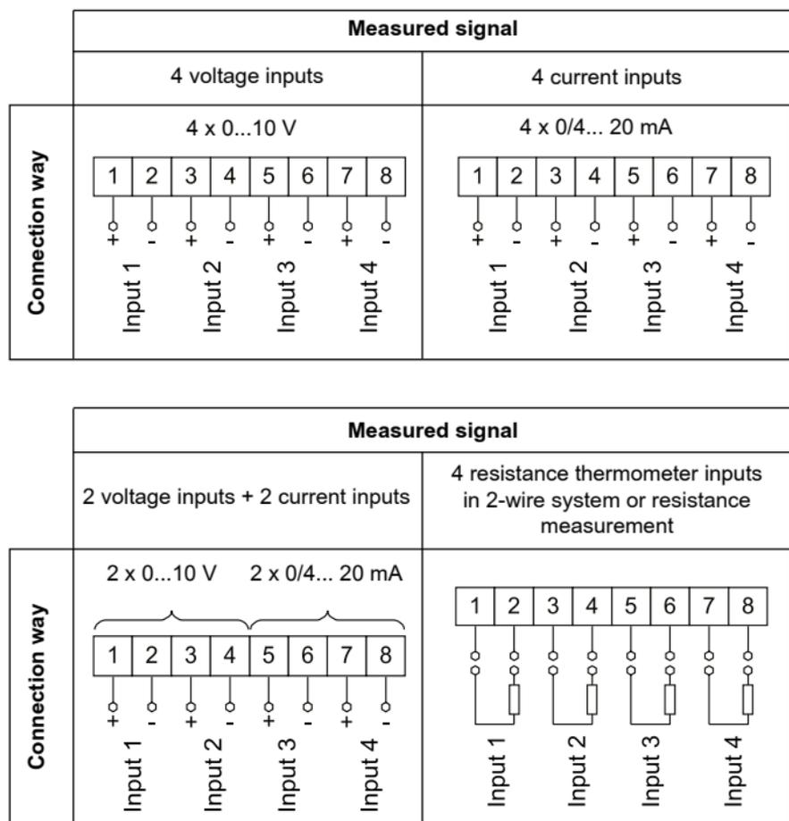
**Fig. 4 connection way of input signals**
